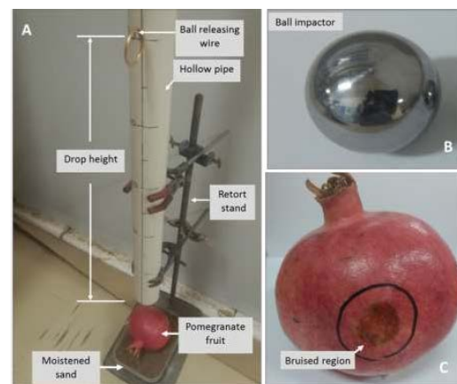
Figure 1 Experimental setup of simulated laboratory bruise impact test (A), stainless steel ball impactor (B), and bruised pomegranate fruit (C)
