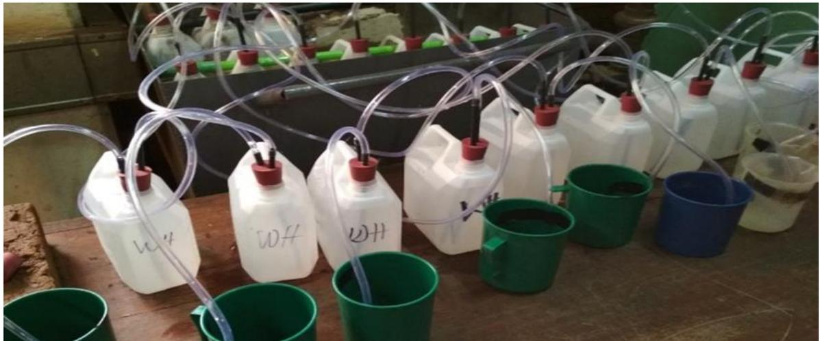
**Figure 1. Actual Biogas production setup**
